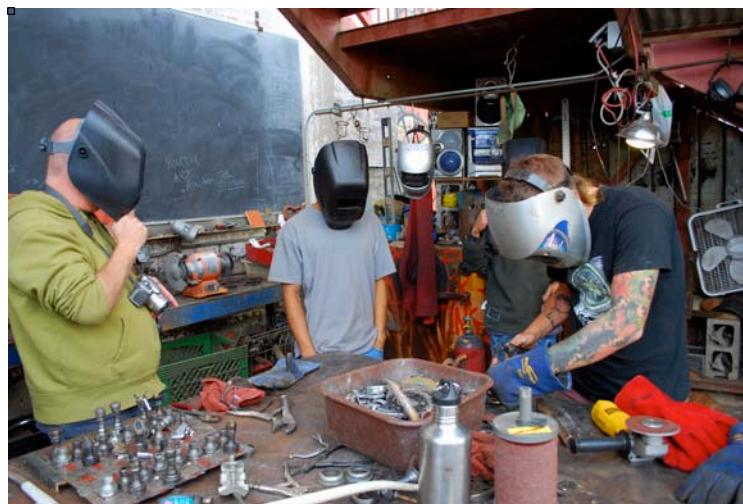
Tucson students and teacher welding recycled bicycle parts to make a bike rack.
